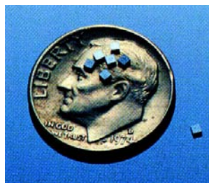
Micromachined Tilt Sensor Element
